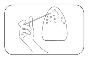
★ Vapour hole on press iron baseplate may be blocked by foreign matters, which requires cleaning by prod often.
